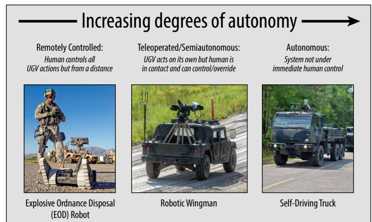
Range of autonomy in unmanned ground vehicles
