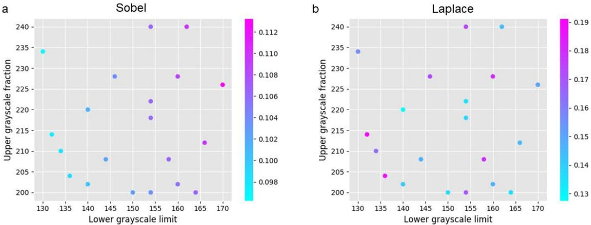
**Figure 8. Estimated graphitic phase fraction (color bar) as a function of thresholding limits for the watershed algorithm using the Sobel (a) or Laplace (b) transforms**
