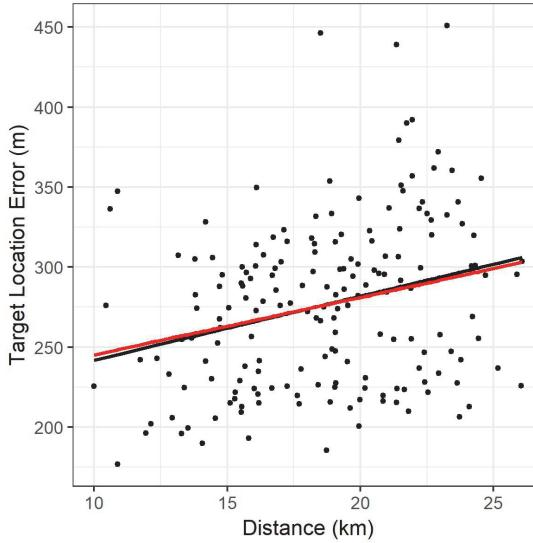
*Figure 5: Linear model fit (black), population level linear mixed effects model fit (red) plotted against full data set. The lines are similar because group-level trends are consistent with population-level trends.*
